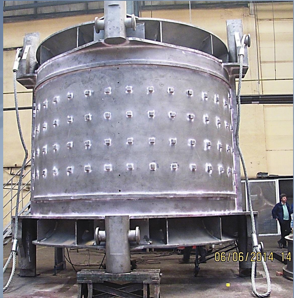
Inner casing 8,7 m 2 for Nuclear Turbine
