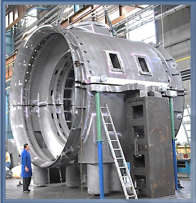
Inner casing 13,9 m 2 for Nuclear Turbine
