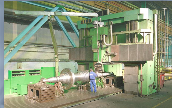
Milling on Movable Portal Milling Machine
